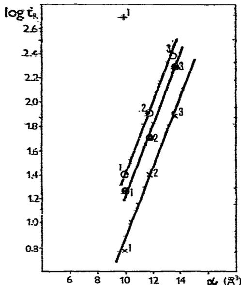
Fig. 1. Dependence of  $\log t'_R$  on polarizability for *n*-alkanes on  $\beta$ -CD at 50°C (O), 60°C (●) and 80°C (x) and on  $\alpha$ -CD at 80°C (+). 1 = *n*-Pentane; 2 = *n*-hexane; 3 = *n*-heptane.
