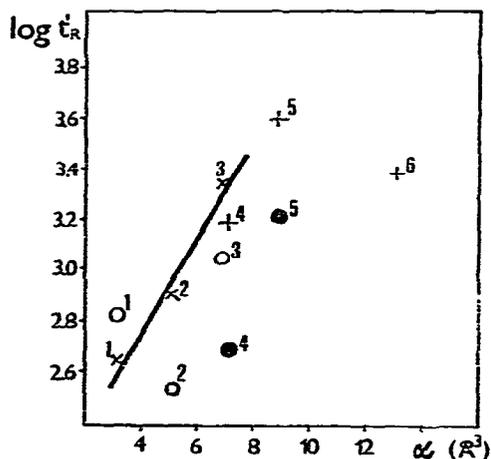
Fig. 4. Dependence of  $\log t'_R$  on polarizability for unbranched (x, O) and branched (+, ●) aliphatic alcohols on  $\alpha$ -CD (x, +) and on  $\beta$ -CD (O, ●) at 80°C. 1 = Methanol; 2 = ethanol; 3 = *n*-propanol; 4 = isopropanol; 5 = isobutanol; 6 = benzyl alcohol.
